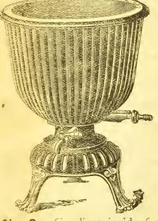
It consists of a corrugated cast-iron case, mounted on legs, with atmospheric gas burner fitted on the bottom of the case. The Boiler is of strong Copper, tinned inside, or best cast iron (which can be supplied rustless by Bower-Barff process), fitted within the case, leaving a space for the hot air from the burner to pass round it, thus economising the gas.
